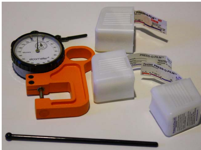
PHOTOGRAPH 5 Testex Press-O-Film Replica Tape (1 January 2017)
