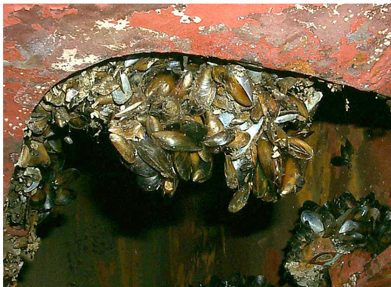
PHOTOGRAPH 3 Mussel Fouling in a Sea Chest
