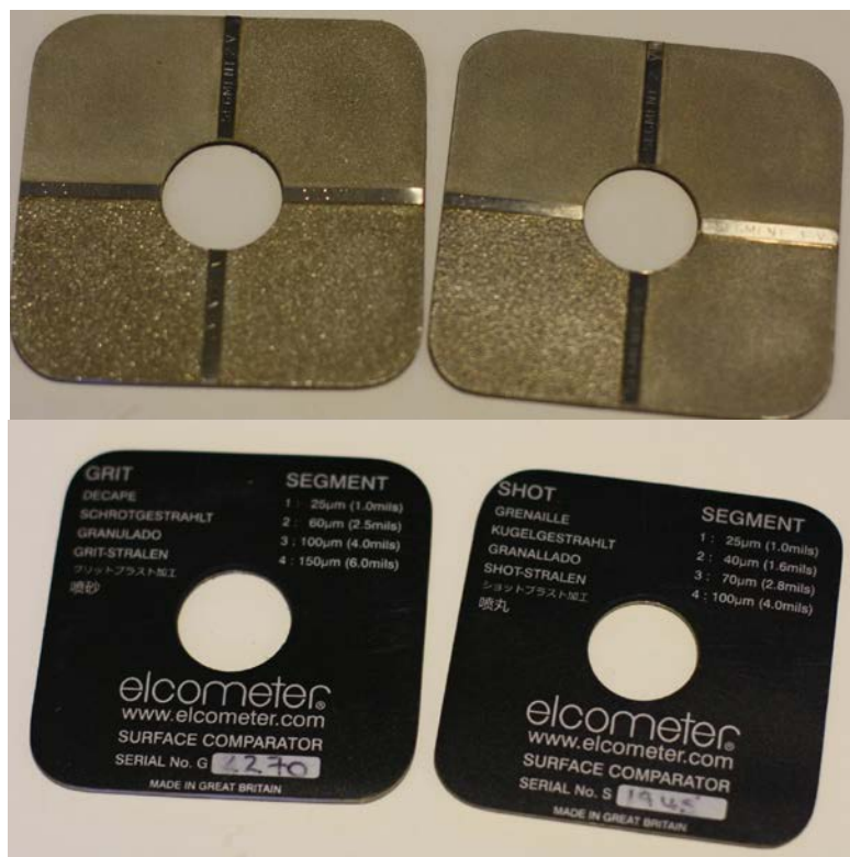
PHOTOGRAPH 3 ISO 8503-1/2 Surface Roughness Comparators (1 January 2017)
