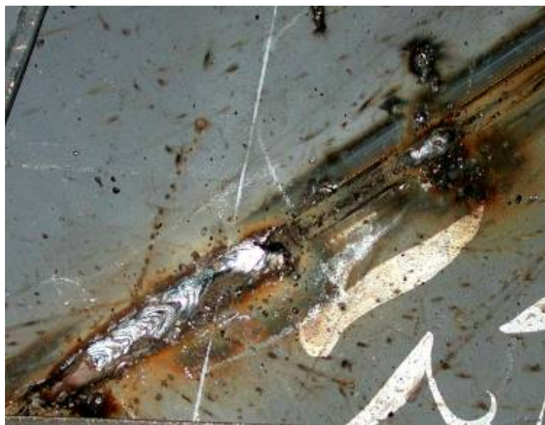
PHOTOGRAPH 9 Weld Fume (Brown Stains) and Spatter
