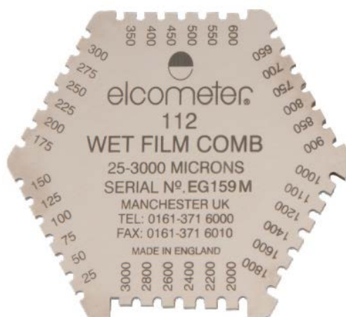
PHOTOGRAPH 2 Wet Film Thickness Gauge (1 January 2017) (Elcometer Coating Thickness Gauge)
