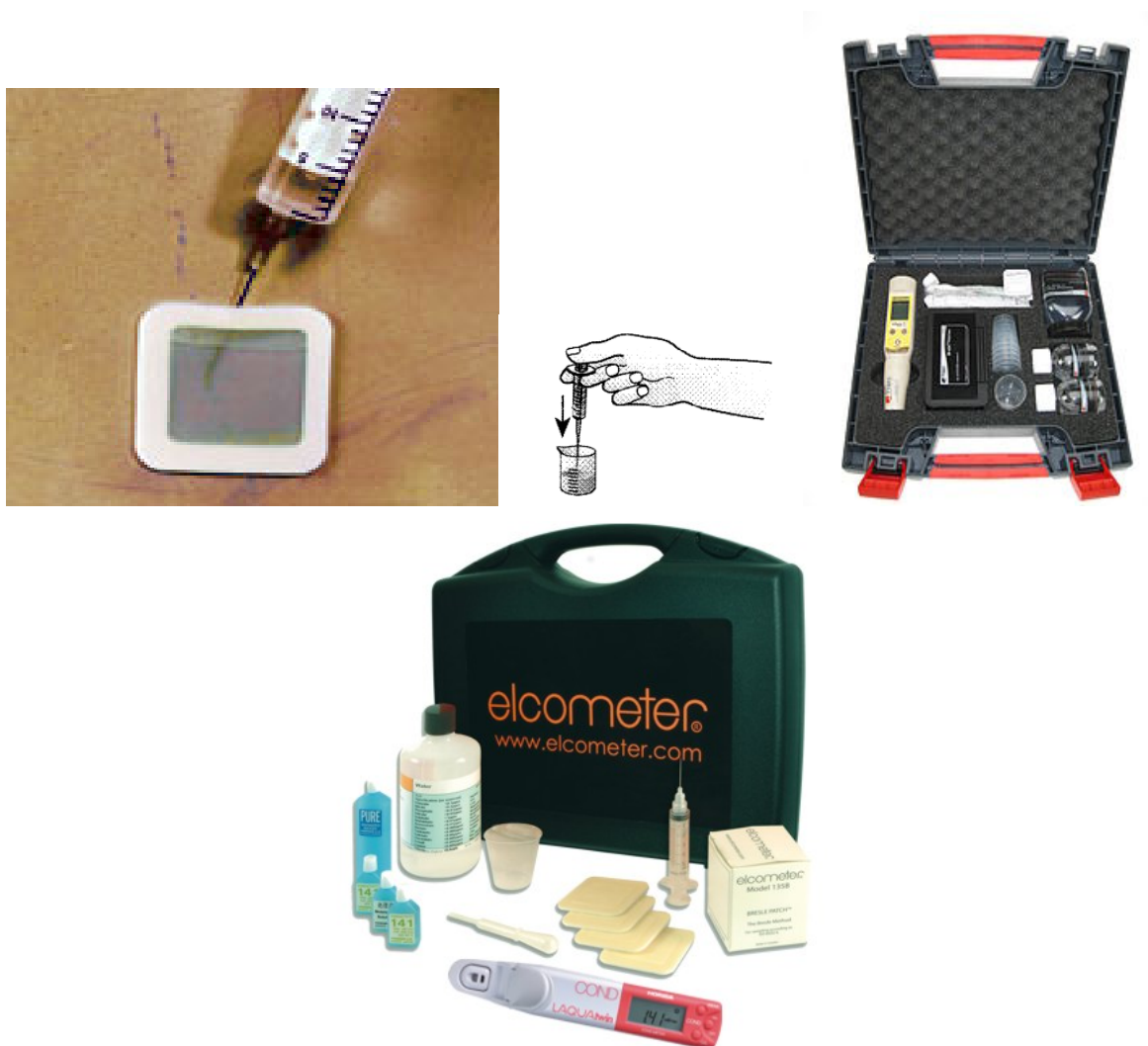
PHOTOGRAPH 9 ISO 8502-9 Compliance Bresle Test Kits (1 January 2017)
