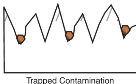
FIGURE 3 Contamination Trapped in the Blast Profile is Over-coated
