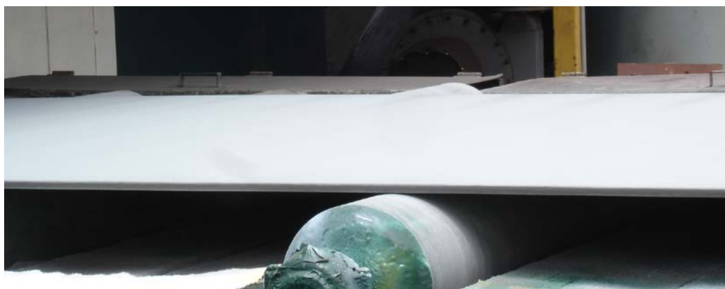
PHOTOGRAPH 12 Steel Plate Coated with Shop Primer (1 January 2017)
