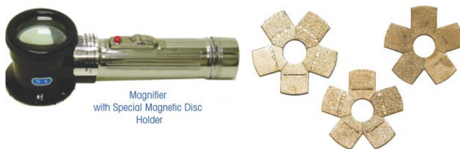
PHOTOGRAPH 4 Keane-Tator Surface Profile Comparator (1 January 2017)
