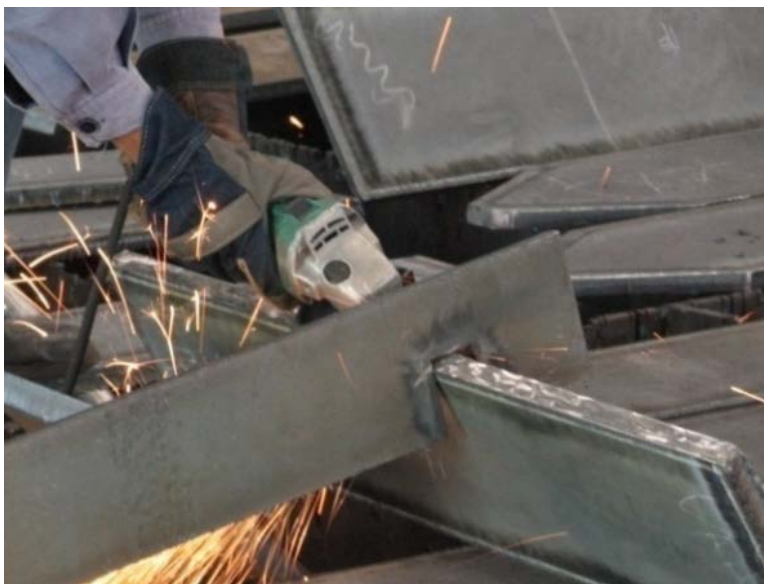
PHOTOGRAPH 13 Edge Preparation (1 January 2017)
