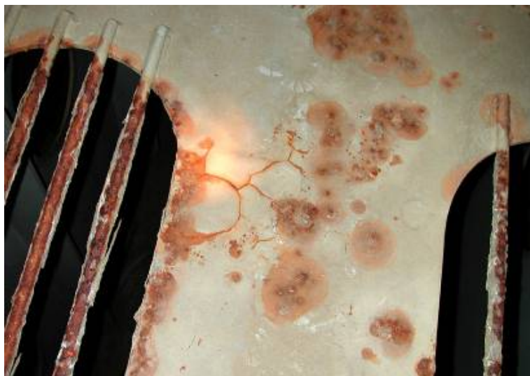
PHOTOGRAPH 24 Typical Mud Cracking in a Thick Coating
