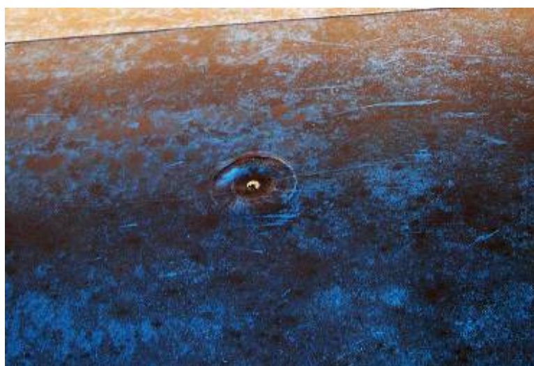
PHOTOGRAPH 6 An Example of a Zinc Reference Electrode on a Ship
