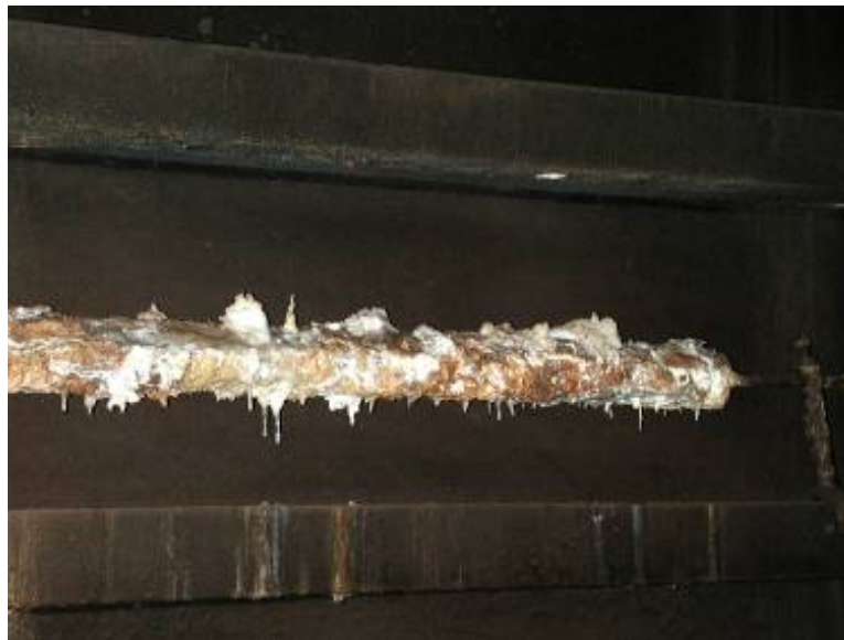
PHOTOGRAPH 3 Overworked Aluminum Anode
