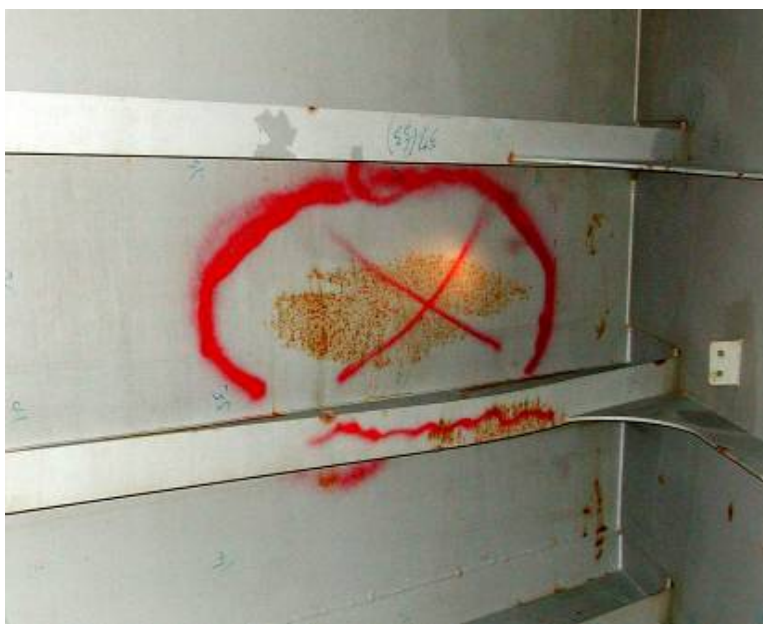
PHOTOGRAPH 23 Reverse Impact from External Collision
