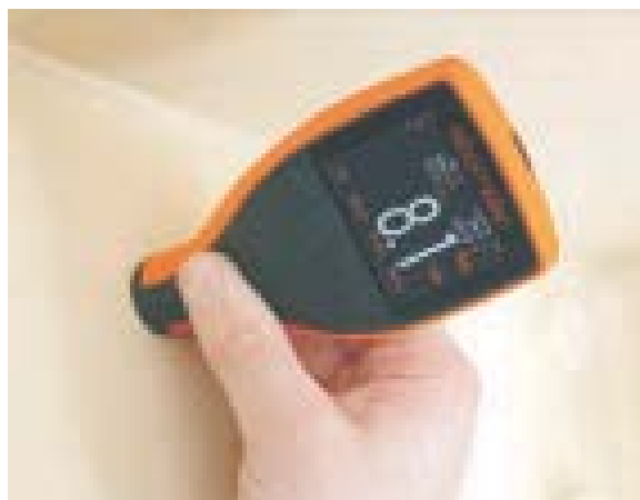
PHOTOGRAPH 1 Dry Film Thickness Gauge (1 January 2017) (Elcometer 456 Coating Thickness Gauge)
