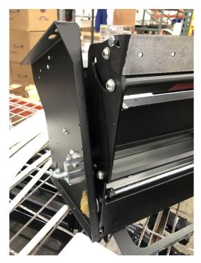
To the left of the step is a manual lock to hold the step in the upper position. This will allow easier access to the motor area on the right.
