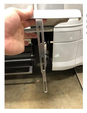
Locate the bracket(s) under the edge of the fiberglass skirt, shown to the left. Remove the screws securing them to the frame, this will allow the fiberglass panel to swing up.
