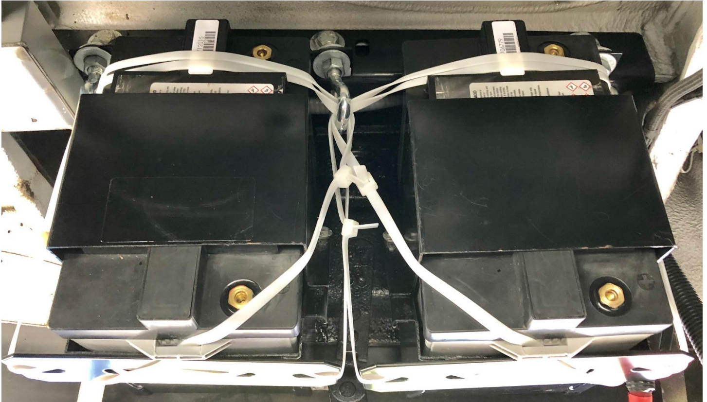
Batteries Reinstalled, Lower Support Plates & Zip Ties Installed & Tightened (Image 4)
