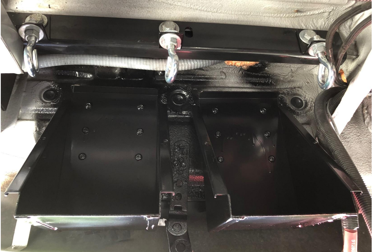
Surfaces Cleaned, Painted & 3 Bracket Eye-Bolt Assemblies Installed (Image 3)
