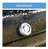
Drivers Side Trays installed, Note 7th rivet in middle of tray. Gray is seam sealer to keep out moisture
