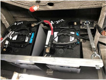
I installed the tray covers but I am not 100% happy with these. The covers do not come together completely due to the taller battery but also because of the molded handle standoffs on the battery. I am going to think about an alternate appraoch to ensure the covers will not loosen while on the road. I am not relying on the aluminum angle to hold the batteries in.
