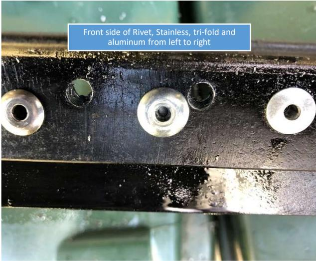
Front side of Rivet, Stainless, tri-fold and aluminum from left to right
