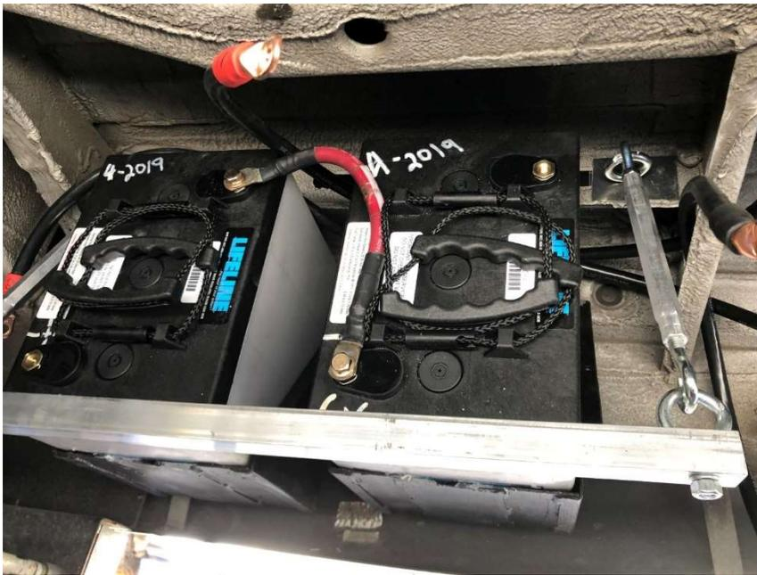
I installed the tray covers but I am not 100% happy with these. The covers do not come together completely due to the taller battery but also because of the molded handle standoffs on the battery. I am going to think about an alternate approach to ensure the covers will not loosen while on the road. I am not relying on the aluminum angle to hold the batteries in.
