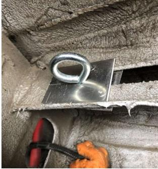
The eye bolt uses two backing plates that capture the rib. Once the batteries were installed, it was gravely evident that the coach sheet metal would flex a very noticeable amount. It is no wonder that these rivets may pull out under the dynamic load of these heavier batteries. Add compromised holes, lower strength rivets or poor riveting techniques and “battery detaches on the highway”.
