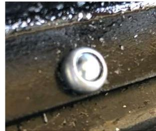
Drivers Side Trays installed, Note 7th rivet in middle of tray. Gray is seam sealer to keep out moisture
