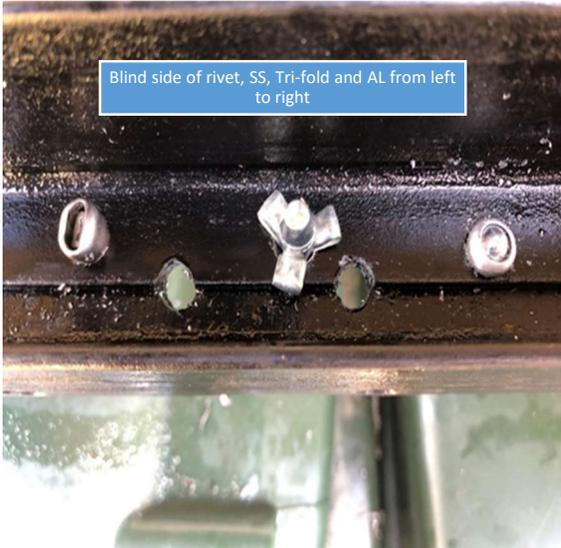
Blind side of rivet, SS, Tri-fold and AL from left to right
