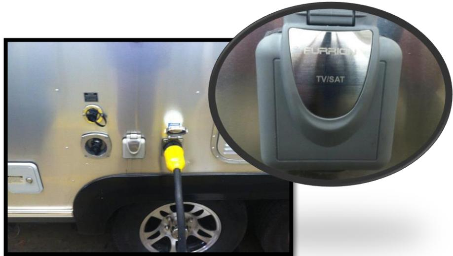
Step 2: Connect your coax from your exterior satellite to the coax connection labelled "SAT"
