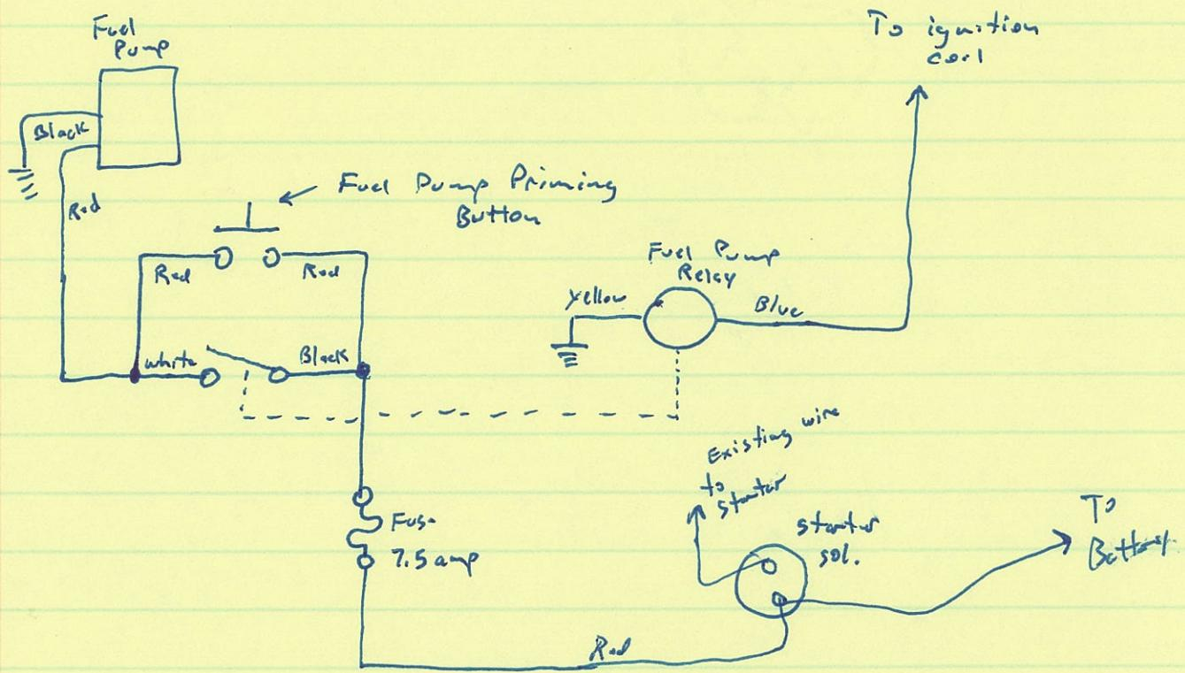
The Fuel Pump Primer Button should be used to pull fuel from the Tank up to the generator if it has ~~setting for~~ ~~setting for~~ a while without being started.
