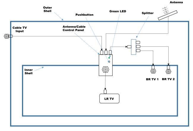
"Stock" Configuration Older Trailer w/o Satellite Wiring
