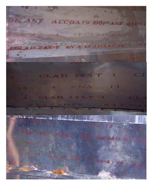
1960's switched to Alcoa for the Aluminum material. Alcoa-Aluminum Alclad sheet 2024-T3 .032
