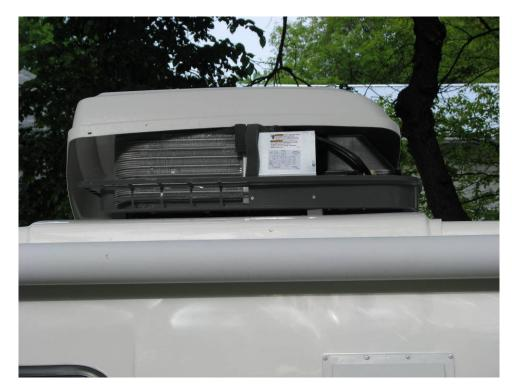
I removed the 4 screws holding the white plastic cover on, one on each side towards the back and 2 on the front using a #2 Phillips screwdriver. I lifted the right side of the cover up and slid it half off towards the left side of the trailer. At the front of the right side there is a metal box with a wiring diagram on the cover that contains the electrical components.
