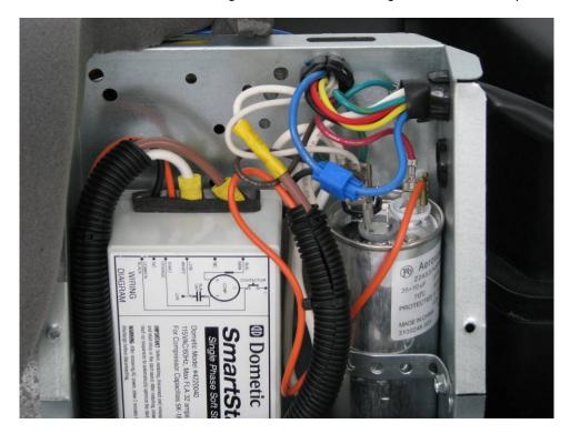
I tucked the wires into the box and reattached the cover by inserting the 2 tabs on the cover into the slots on the box and then fastened it in place with the 2 screws. I reattached the sticky backed foam that I had removed earlier to get at the screws.
