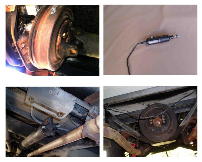
A Dremel tool (pictured) was used to score marks on the components. This would be so that they could be oriented the same way on replacement. It turned out the drive line shop assumed each component would have been individually balanced. They didn't think it would be necessary to balance the drum and shaft together after shortening the shaft. So the marks really weren't of any use.
