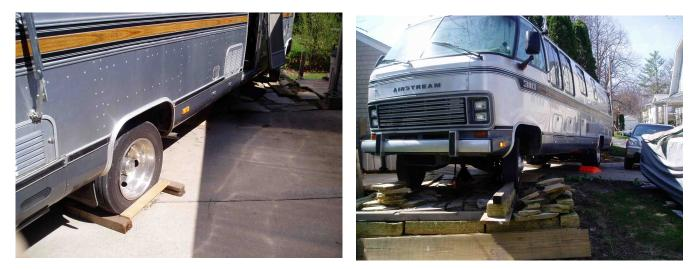
The hydraulic jack was adequate to bring the coach's front wheels off the ground so it could be supported by the two 12,000 pound stands (below left).
