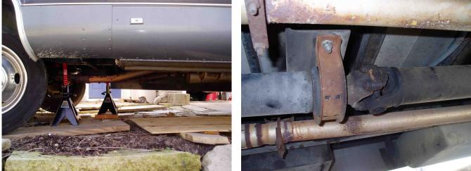
The next photo shows the carrier bearing between the first and second drive shafts. I partially dropped the carrier bracket and tied wire to the second shaft to keep it from dropping down.
