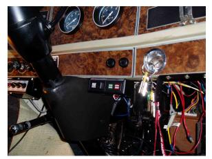
Next the dash console was mounted. I used nuts and stove bolts because the dash is plastic and would not hold up to sheet metal screws. It was a little bit of a chore because there was a piece of metal bracket on part of the site—I modified the supplied shim and added a spacer on one side so the console is level under the dash.
