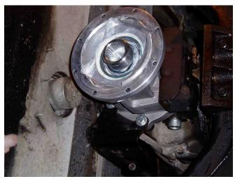
After shimming the coupler and replacing the transmission mount, it was time to mount the Gear Vendor unit itself!
