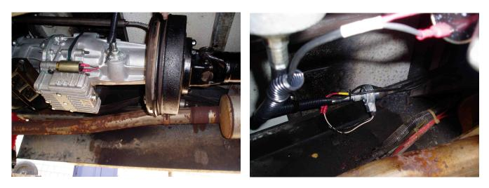
I put a bracket between the speedometer gear and the sender to pull the cables away from the exhaust pipe. Also tied up the slack cable under the dash.
