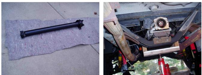
cable and the speedometer cable and the bolts holding the rubber transmission mount. The Talcott Automatic Transmission Jack is deployed. I then removed the tail assembly (six bolts), and the rubber transmission mount (two bolts).
