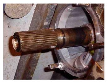
GV is sending a new coupler and I am burnishing the shaft where the splines are mushroomed and distorted, mainly out towards the end. Here's the "before" picture....
