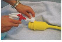
2 Apply soap solution to shoulder of boot (plug side) and to rear opening of ring.
