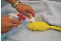
2 Apply soap solution to shoulder of boot (plug side) and to rear opening of ring.
