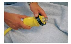
3 With a twisting motion, force ring **past** shoulder of boot. (Use same procedure for connector.)
