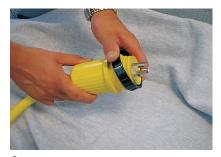
3 With a twisting motion, force ring **past** shoulder of boot. (Use same procedure for connector.)
