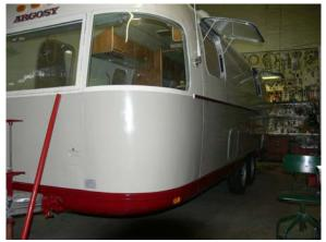
Enclosed belly pan was then topped with Burgundy epoxy paint to a ¼" above the belly pan molding to keep water from entering behind the trim molding. The beltline insert has presented some problem for us in duplicating the color. Originally I have considered using Formica strips
