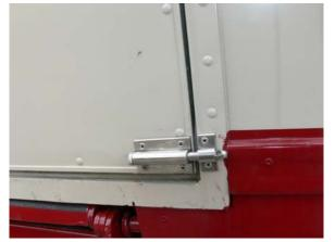
In order to positively secure the door from opening during towing a stainless steel bolt was fabricated. End of the slide bolt has a hole drilled across for the padlock.
