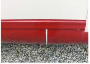
The belly pan wrap joint is only  $\frac{1}{2}$  wide on the outside.
