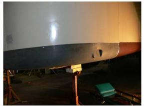
Front aluminum panel of the belly wrap was inserted over the top edge of the banana wrap to prevent the water from the road from being forced into the belly pan during towing.
