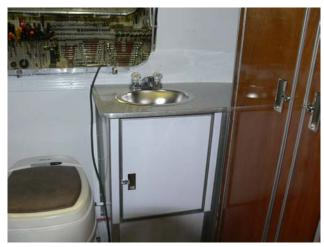
Bathroom has a lightweight SS sink atop of homemade cabinet with a Formica countertop which was trimmed with ¾" anodized aluminum T trim. Walls of the cabinet are NUDO Panel [Aluminum clad corrugated Vinyl clad plywood substitute]. Bathroom linen closet houses all electrical panels and the INTELLIPOWER 9200 with charge wizard. 110 Volt circuits are protected by GFI breakers.
