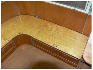
Seat bases are 3/8" varnished plywood and are removable to gain access to underside.
