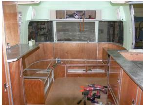
Looking from the rear to the front, a wrap around sofa base was framed out of TIG welded aluminum angle with a side table on the right side.
