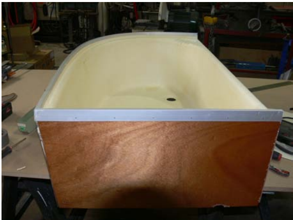
Face panel with aluminum H trim joining it to the tub.
