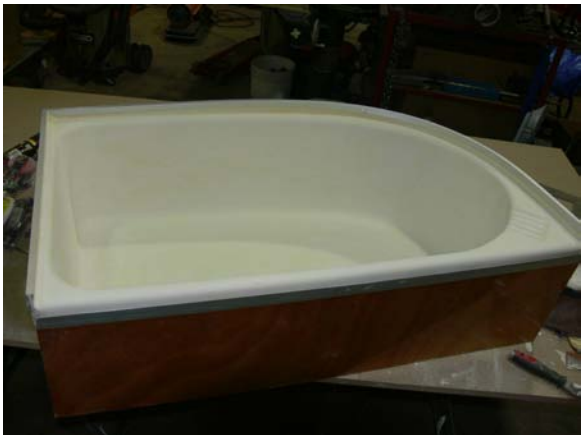
Face panel with aluminum H trim joining it to the tub.
