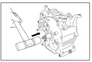
FIGURE 69. CRANKSHAFT REMOVAL
