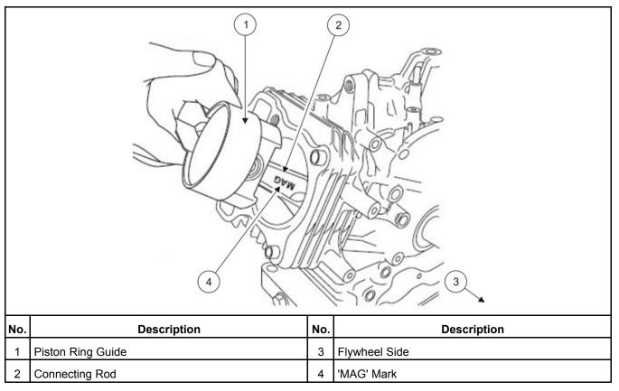
FIGURE 65. CONNECTING ROD ASSEMBLY
