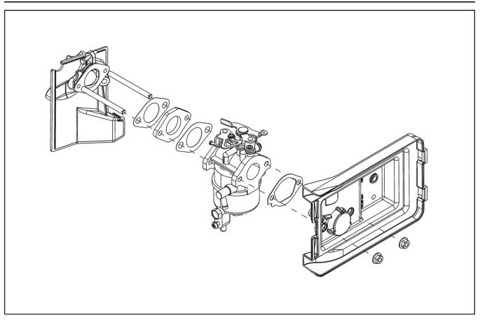
FIGURE 25. CARBURETOR AND INTAKE MANIFOLD ASSEMBLY
