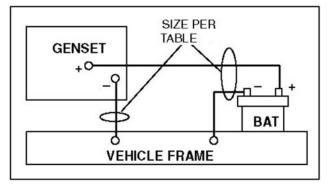
FIGURE 11. VEHICLE FRAME AS PATH FROM BATTERY NEGATIVE (-) TERMINAL
