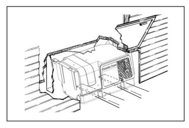
FIGURE 4. COMPLETE GENERATOR SET REMOVAL
