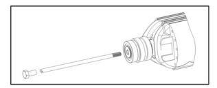
FIGURE 15. ROTOR REMOVAL
