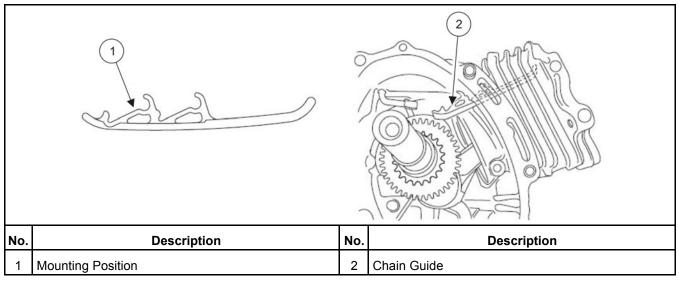
FIGURE 56. CHAIN GUIDE ASSEMBLY
