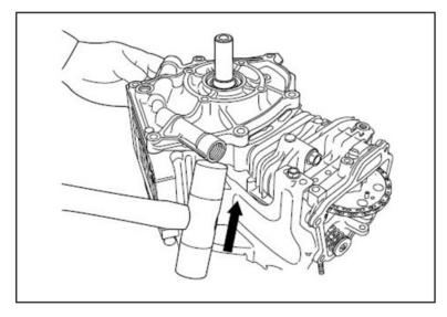
FIGURE 48. MAIN BEARING COVER REMOVAL
