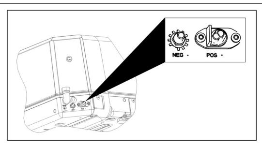
FIGURE 12. BATTERY CABLE CONNECTIONS
