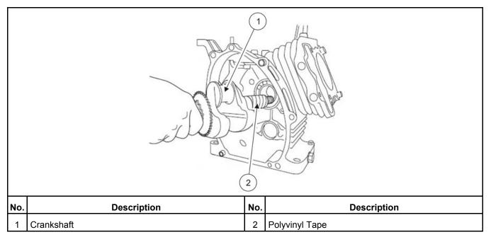
FIGURE 70. CRANKSHAFT ASSEMBLY
