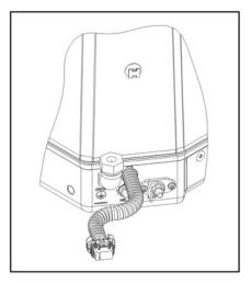
FIGURE 9. 8-PIN CONNECTOR
