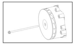
FIGURE 13. ALTERNATOR BOLT
