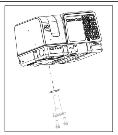
FIGURE 21. SPARK ARRESTOR
