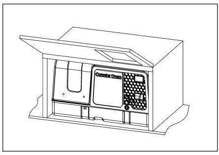
FIGURE 2. TYPICAL COMPARTMENT MOUNT INSTALLATION
