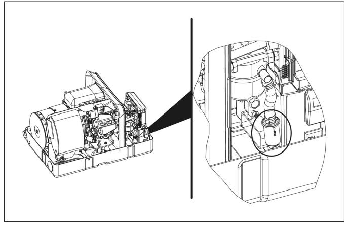
FIGURE 28. FUEL FILTER REPLACEMENT
