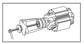
FIGURE 19. ROTOR BEARING REMOVAL
