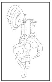
FIGURE 32. LPG CHOKE ASSEMBLY
