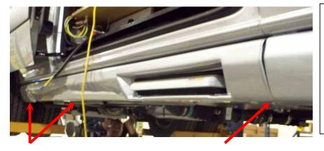
**Step 1:** Remove the pop rivets from the outer fender flairs to allow for mounting of the new brackets.
