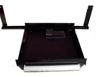
Simply start by removing original Thule step. You will need to lift the interstate into the air and coming from the underside removing all fasteners and brackets at the rear of the step and from behind the flare. Disconnect the wires going to the step leaving enough wire to connect into the new Project 2000 in the process below.
