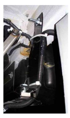
Step 2: Install front rear mounting bracket to the structure on the underside of the chassis on main frame rail.
