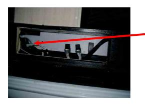
Mounting location of the electronic step controller. This is behind the clack close out. Remove 6 screws to gain access.
