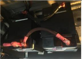
Connect additional AGMs to existing OEM house batteries. NOTE: The connection shown is not optimal for battery life or balance, but selected in this experiment to avoid additional cable length (and associated voltage drop) from the Passenger Side to the Driver Side.
