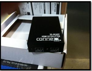
Note: If your unit only has 1 TV it WILL NOT have an HDMI Splitter. The output HDMI from the Blu-Ray will run directly to the TV. This will become the output for your new HDMI splitter and you will need new HDMI cables for your Blu-Ray and Satellite Inputs.
