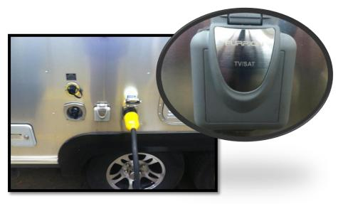
Step 2: Connect your coax from your exterior satellite to the coax connection labelled "SAT"
