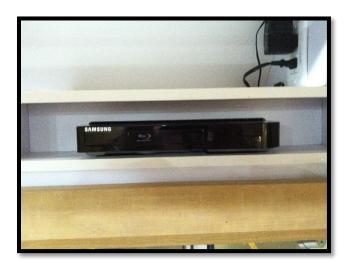
Step 4: Disconnect the Blu Ray player and remove the 3 phillips head screws in the Blu Ray box and remove the box. Some models may have the box attached with velcro as well.
