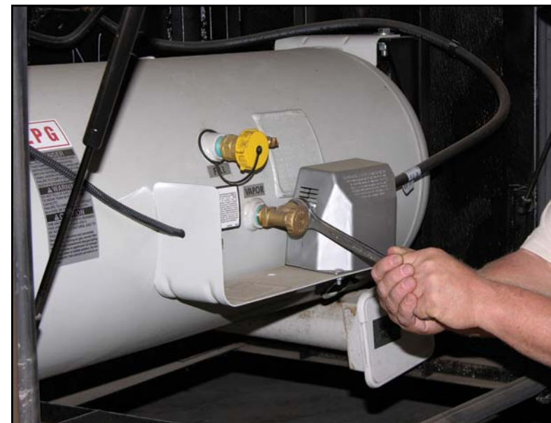
Professional RV technicians keep a variety of different size flare plugs and caps (above) to use when locating propane leaks. RV owners can check for propane leaks by spraying a soapy solution on fittings (left) to see if bubbles appear. Avoid using solutions that contain ammonia or chlorine products because these can damage fittings.
