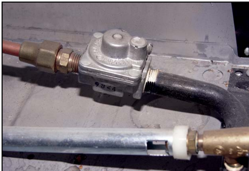
Many of today's more efficient appliances require less operating pressure, and have additional "third stage" regulators, like this one on the fuel inlet fitting to an RV range/oven.
