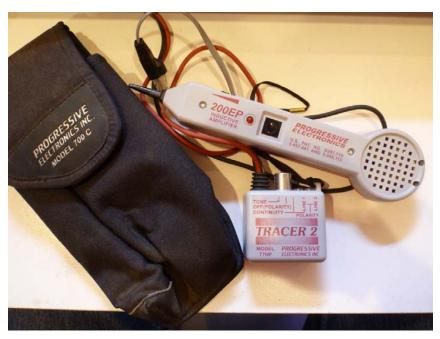
A typical signal tracer set consisting of a tone generator/continuity tester (small box marked "Tracer 2") and signal tracer amplifier/'banana' (marked 200EP.)
