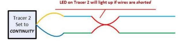
When checking any two wires to see if they are improperly shorted together remove any light bulbs, LEDs, or other devices from the wires and as always turn off the power just to be sure you're measuring only the wires and not what is attached to them.
