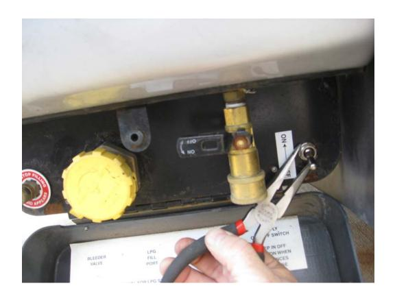
Remove the old switch by using needle nose pliers.
