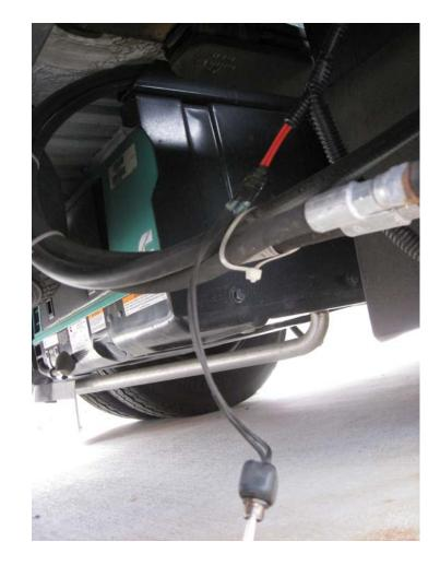
Connect the two new wires to the old two red wires using crimp connections or solder. I soldered and then used shrink tubing to insulate them, and then zip tied the as far up into the chassis as I could to the existing wire bundle. Also, place the wire as far as you can in the black wire wrap to protect it as well.
