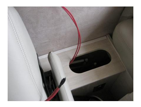
Pull the wires from under the seat, to the area under the cupholder. Here, the wires are shown after I pulled it. Note they will not come up through the cupholder. You may want to remove the rear couch for the next step.
