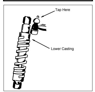
b. **To shorten unit:** Grasp lower casting firmly and tap bottom mount with hammer. This will cause shock barrel to slide into casting to desired length.
