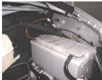
Aux Battery located in engine compartment
