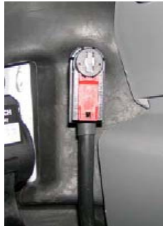
Unhook Vehicle Ground Located next to accelerator pedal
