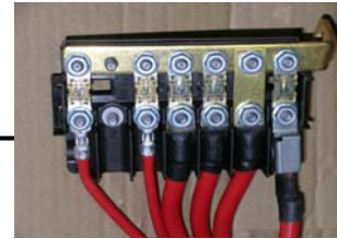
Pre-Fuse Box located on battery (+) pole
