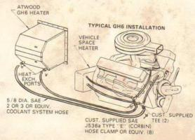
Above is a "typical" GH6 installation. For best results use a 160° thermostat in the summer and a 195° thermostat in the winter.
