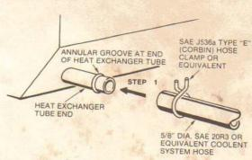
Push hose end (with clamp attached) onto tube end as far as possible.
