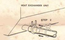
STEP 2 Spread hose clamp and slide toward heat exchanger unit: past annular groove and release.
